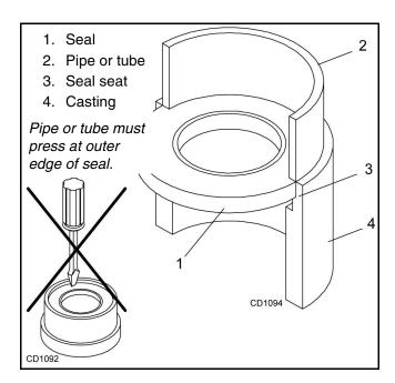
Figure 17. Seal Installation
